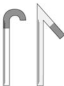
Pipeline casing vents
